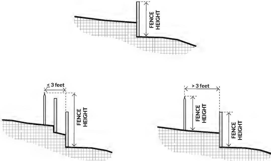
FIGURE 18.02.030.C.1: MEASURING HEIGHT OF FENCES OR WALLS
