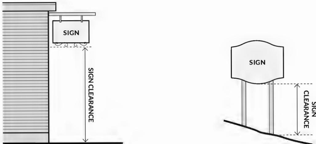
FIGURE 18.18.050.C: MEASURING SIGN CLEARANCE
