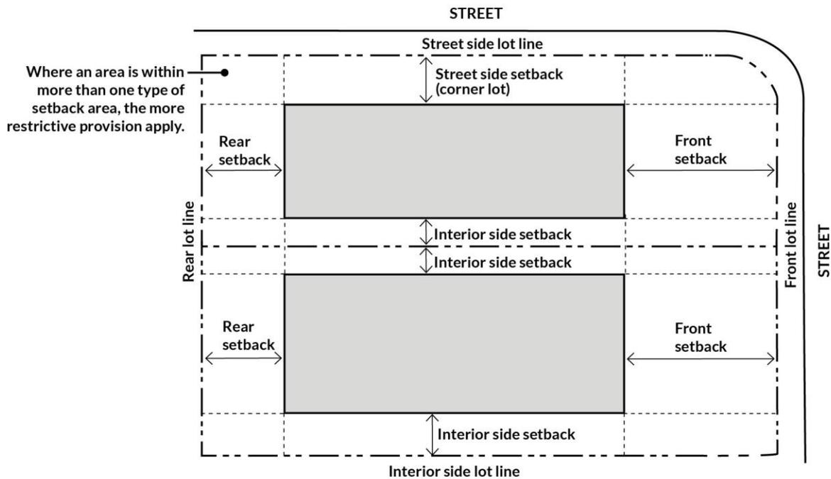
FIGURE 18.02.030.I: DETERMINING SETBACKS
