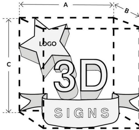
Sign area is computed using the smallest rectangular prism that will encompass the entire sign.
